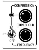
Turn on the Compressor by selecting the 3:1 position on the face panel of the M-2000. With the Threshold set per the example to the left, play a low note and sweep the Frequency control clockwise.
